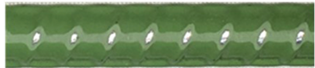
(b) FBE coated steel with scratch damage to the coating
